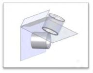
Note: Tilt The Vision Pro adaptor up as shown to set into place, then swing down to meet flush with the opening in the drawer.
