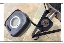
Step 3 – Clip the pit probe to the top of the cooking grate inside your cooker and turn the power switch on. Adjust the setpoint using the UP ▲ DOWN ▼ keys.
