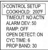
Scroll through values in the CONTROL SETUP SCREEN using the UP/DOWN keys. To modify a value press the M/E key. Use the LEFT/RIGHT keys select the digit to be modified. Adjust the value with the UP/DOWN Keys. Press the M/E key to save. To return to the MAIN SREEN press the UP and DOWN keys together.
