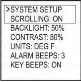
When SYSTEM SETUP is in the top line (with arrow) pressing the LEFT or RIGHT key will index to the next or previous setup screens (see menu diagram).
