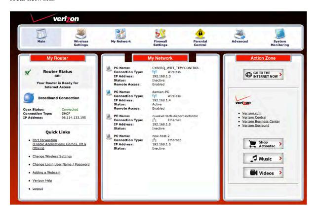
Create a new port forwarding rule by selecting CYBERQ\_WIFI\_TEMPCONTROL under the "Specify IP" dropdown and select "HTTP" under the application dropdown. Then click Add and then click Refresh and it should now appear in the list. Note that the CyberQ Wifi's IP address (192.168.1.3) was assigned to port 80. 80 is the default port number used by all web browsers to get web pages using HTTP (Hypertext Transfer Protocol).
