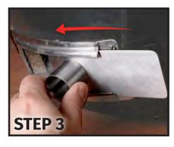
Using the Draft Inducer Sleeve as a handle, slide the Adaptor Door all the way to the left.
