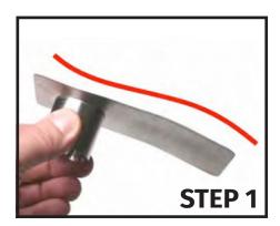
The Grill Dome Cooker Adaptor Door should be bent generally in the shape of the red line to cause it to seal tight in the track. You may shape the door to fit your needs.
