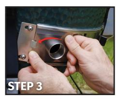
While holding the Expansion Clip in place in the top track, grip the inducer sleeve and pull down until the Adaptor Plate engages the bottom track. Push the Adaptor Plate to the left and under the stop tab.
