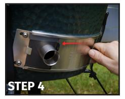
Close the original manufacturer's draft door OVER the top of the Adaptor Plate until the leading edge touches the Draft Inducer Tube and the expansion clip moves all the way to the left. (Reverse order to remove.)
