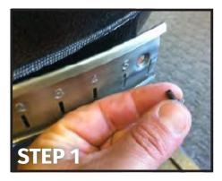
Remove the right screw from lower Damper Track.
