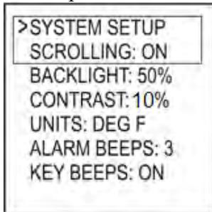
When SYSTEM SETUP is in the top line (with arrow) pressing the LEFT or RIGHT key will index to the Control or Wi-Fi setup screens.
